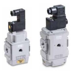
Parker Global Series Combined Soft Start/Dump Valves, provide for the safe introduction of pressure to machines or systems. Soft Start/Dump Valves when set, allow the pressure to gradually build to the set point before fully opening to deliver full flow at line pressure.
